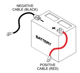
**Figure 5. Battery Cable Orientation**
